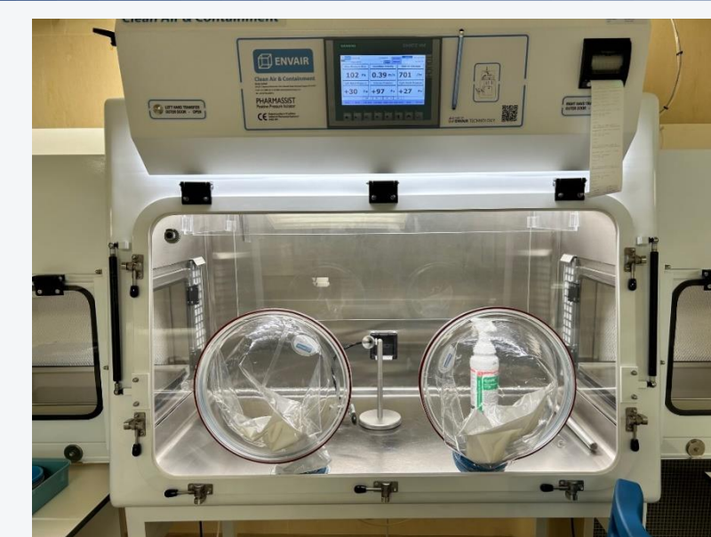
Figure 5: Setup for gassing cycle in Envair Isolator
