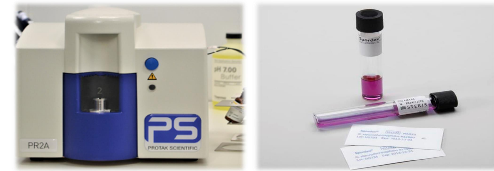
Figure 2: (A) PR2A Luminometer for EI analysis, (B) Spordex Broth & BI strips pre- VHP exposure.
